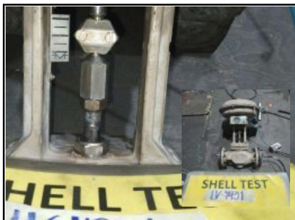
Shell Test (As Left)/No visivle leakage
