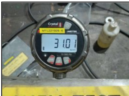
Shell Test (As Left)/No visivle leakage
